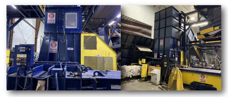
The pre-press lid increases the input density of each charge, reducing the number of strokes to make a bale increasing production by 40% over traditional 2rams without lids. As the lid compresses, material pre-charges in the hopper above the lid – creating the perfect charge for the next compression. The Bale Tie Option provides the production advantage of compacting on the second bale while the first bale is in tie process – increasing production. Fastest 2ram baler in the industry.
